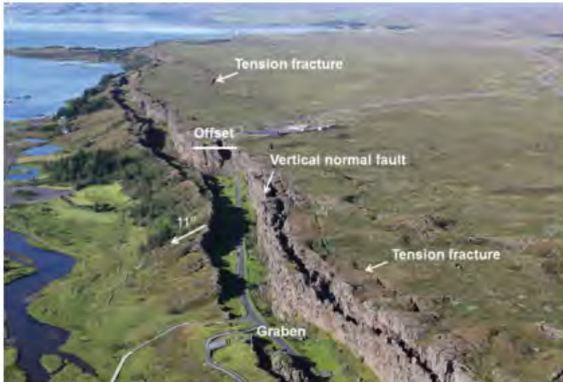
Fig. 5.8 Aerial photograph showing some of the main structures associated with Almannagjá. Around Almannagjá itself there are many smaller structures. These include small tension fractures (discussed in detail in connection with Figs. 5.11, 5.12 and 5.15) and the inclined eastern fault wall (its surface is inclined by 11^\circ to the east, as shown here). By contrast the surface of the western fault wall is horizontal. Where you enter and start your walk down Almannagjá, one segment or part of Almannagjá is ending laterally (as a tension fracture). Then there is an east-west offset (indicated) and a new segment takes over and continues to the southwest. While Almannagjá is a gaping or open normal fault, its opening is so large (more than 60 m in places) that it resembles a narrow graben (indicated). Compare the vertical section in Fig. 5.9
